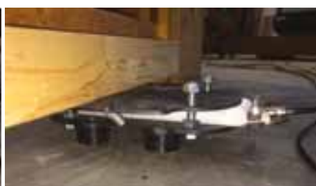
Deflate brake to move scenery freely. The plates on either side of the pneumatic pillow are held in place with a lateral spring to keep the plates together so that they don't come into contact with the floor when deflated.
