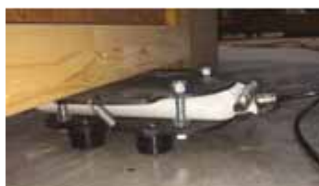
Fill with air to lift your piece of scenery so it will not move
